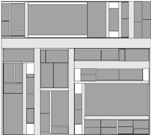
Figure 8: Layout for ami49 (area: 57.3\text{mm}^2 )
