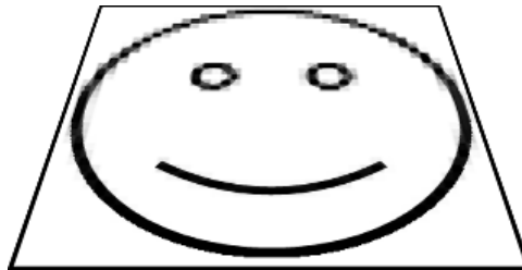
Figure 2.26.: Blending mipmaps when the quad is depicted in perspective.
